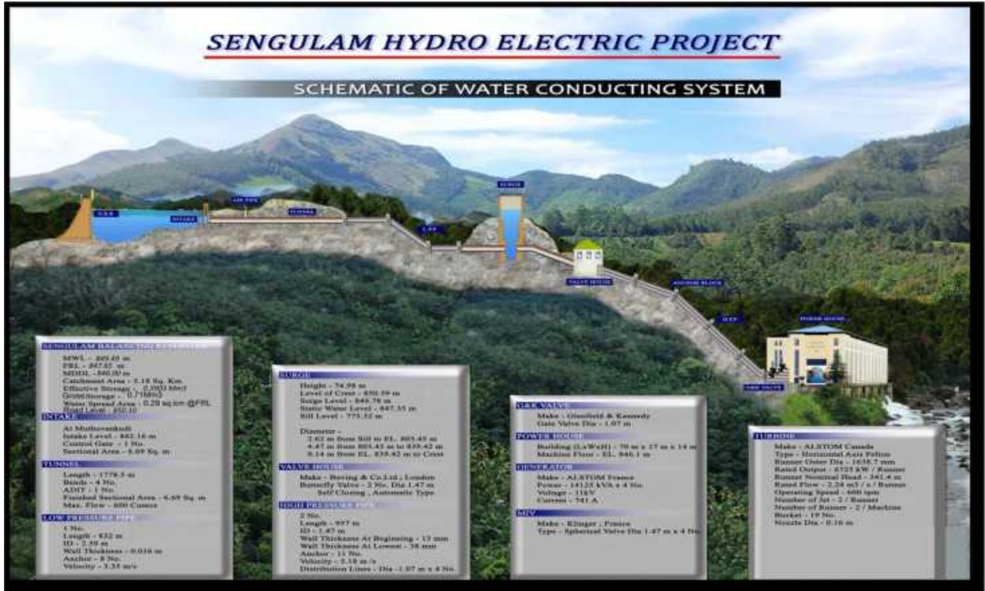
Fig 1.5 Longitudinal Section of the water Conductor System of Sengulam HEP from SBR to Power House
