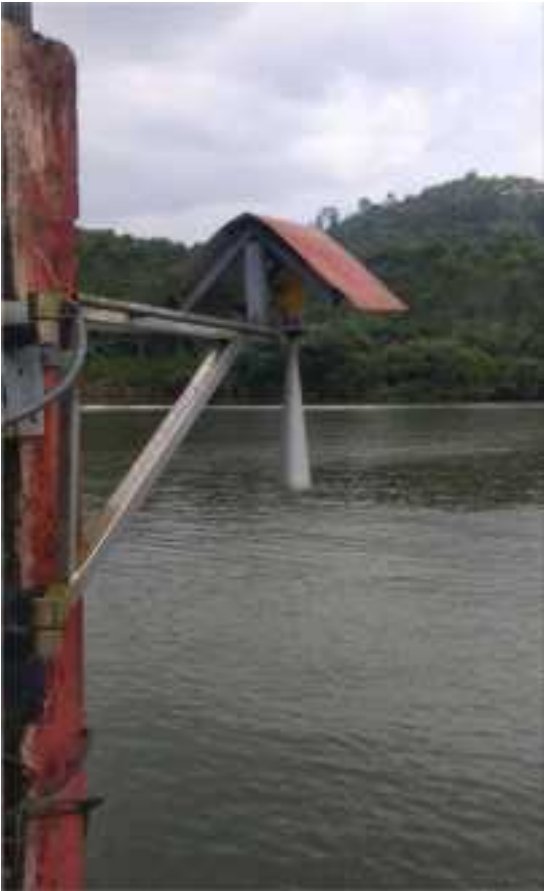
Fig 6.2 Photograph showing Automatic Water level recorder
