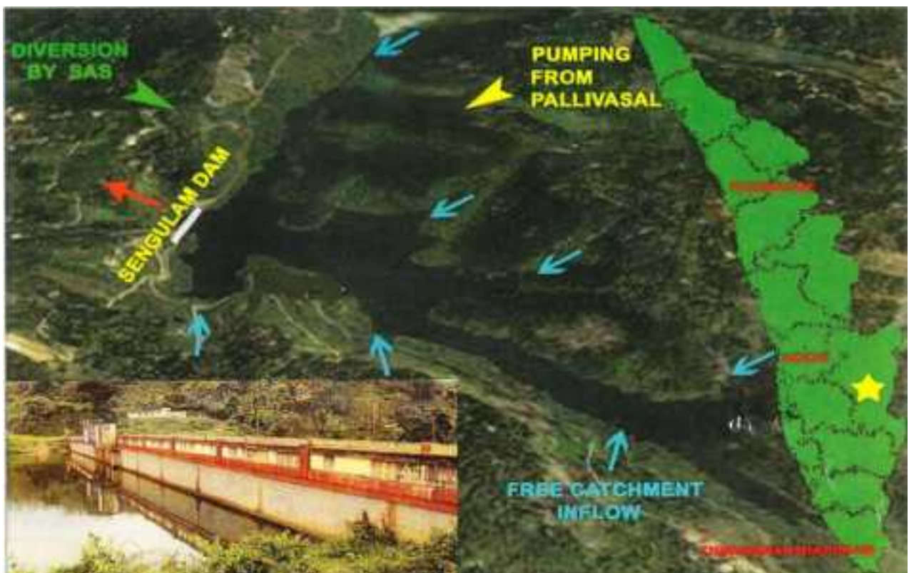
Fig 2.5 Inflow details of Sengulam Balancing Reservoir
