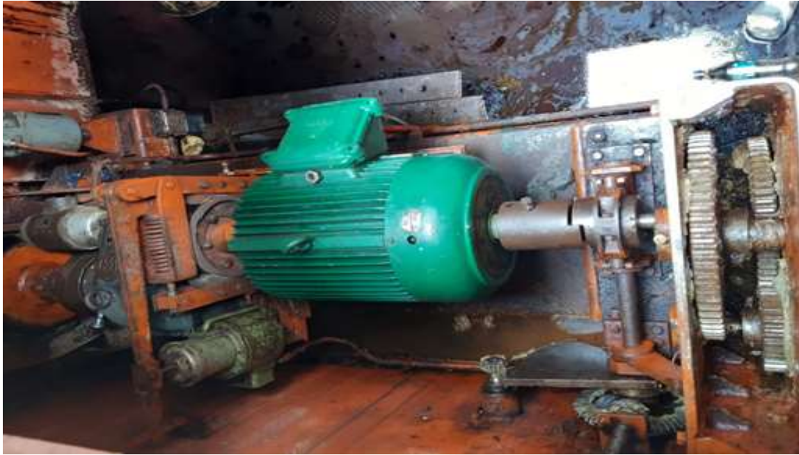
Fig 2.18 Motor of opening arrangement of disperser valve
