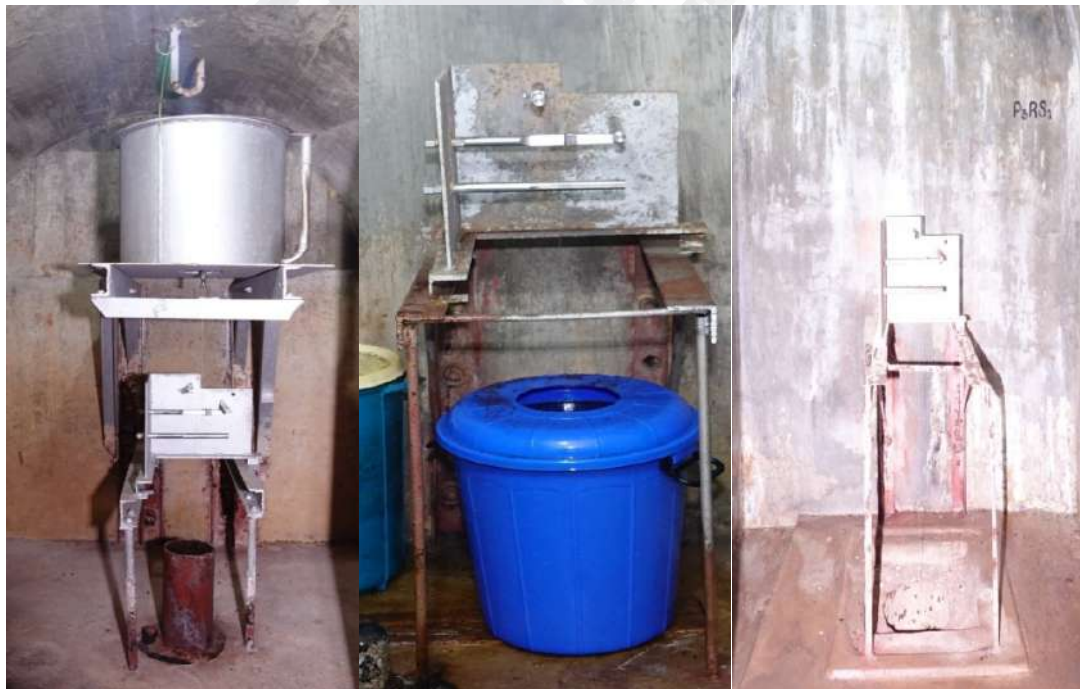
Fig 5.7 (a) Inverted Pendulum (b) Pendulum Station (c) Reading Station
