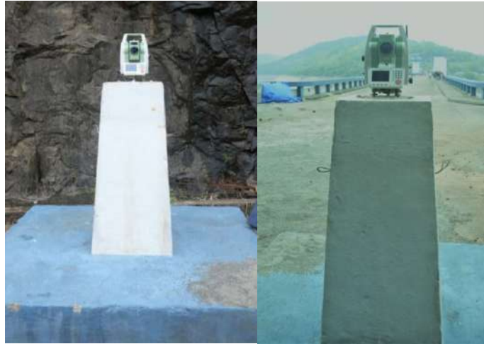
Fig 5.6b Instrument station for crest collimation at right bank
