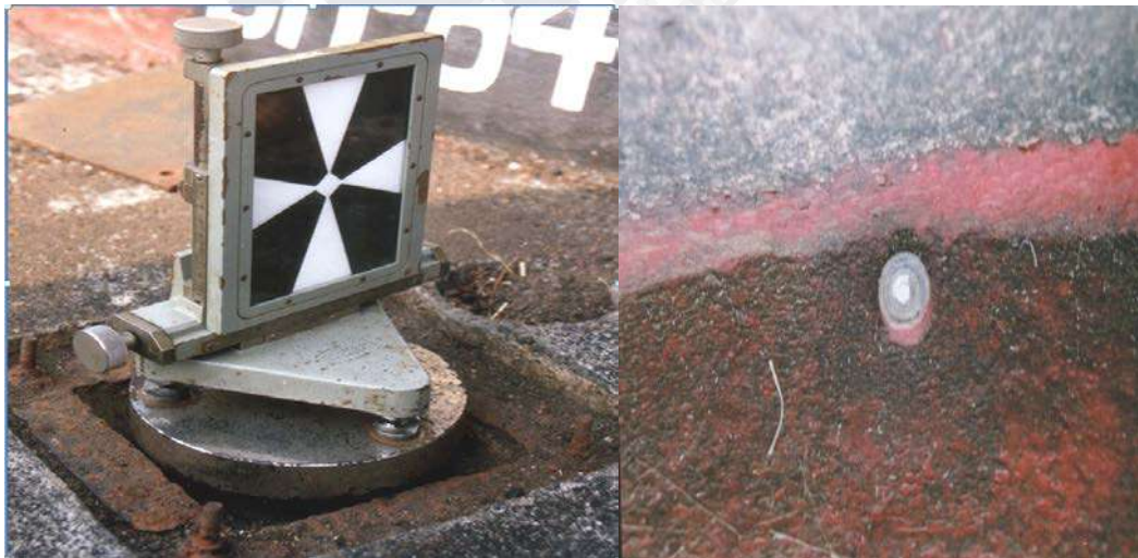
Fig 5.3 Mobile Target and Fixed Target for Crest Collimation
