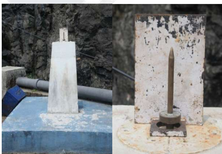
Fig 5.6a Reference monument station for crest collimation at left bank
